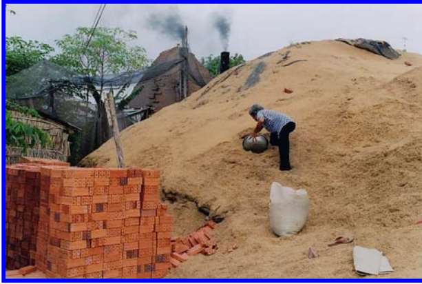
Figure 7 – Rice Husk stockpile at small kiln
