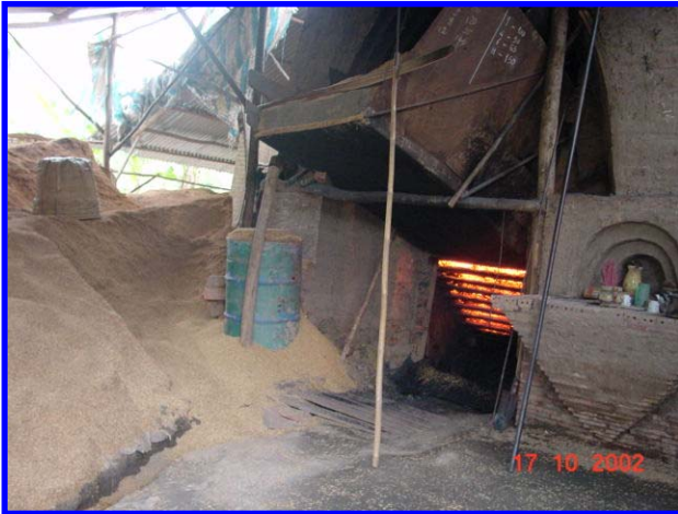
Figure 8 – Rice Husk/Wood kiln
