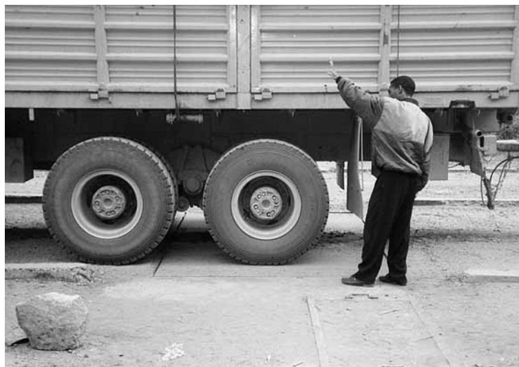
Figure 5b Axle on fixed weighbridge
