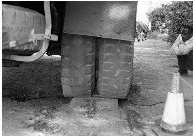
Figure 7 A narrow weighpad may be a safety hazard
